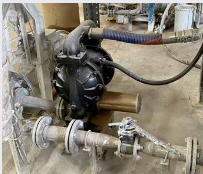
High suction lift reduces pump delivery.
